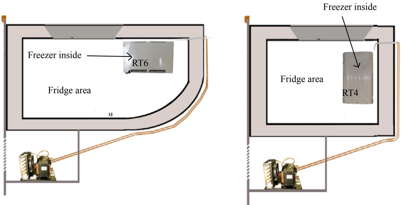
RT4, R26 and RT6 can be mounted vertically or horizontally to enclose a small freezer inside a larger fridge area.
