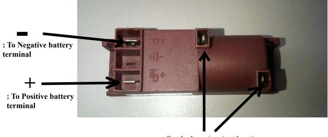
Spark plug wires (not location specific. unused terminal to be grounded
