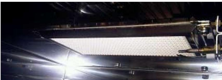
The Bezel secures the burner to the oven roof and protects the ceramic grill as the oven expands and contracts in use.
