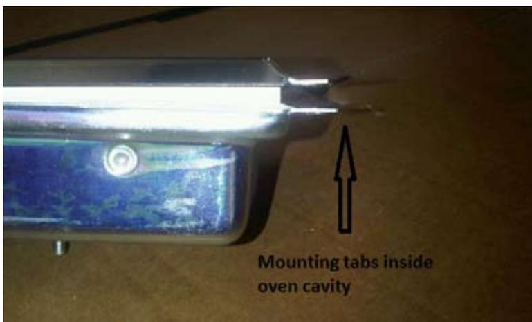
The burner is positioned with the body and throat of the burner in the cavity between the oven roof and the top tray. the mounting tabs and Bezel are inside the oven.
